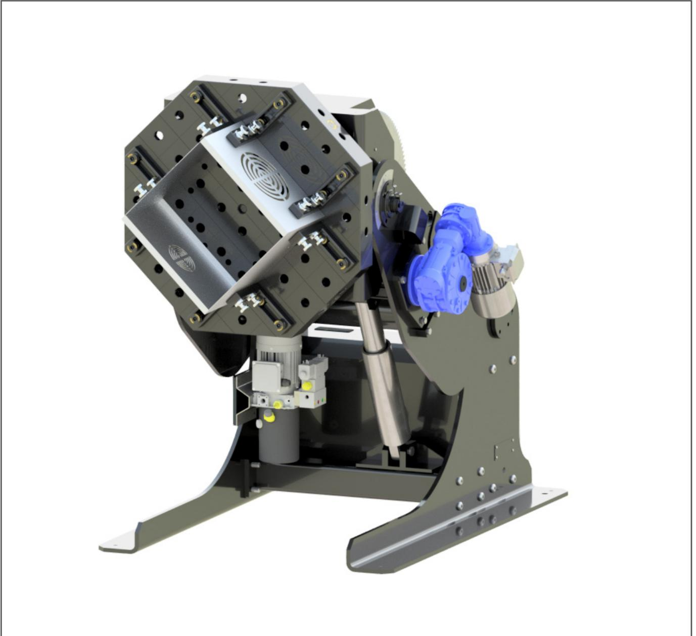
**Octagonal tabletop, installed on TWELVE-3D positioner, in this example is suitable for fixing a sheet metal structure.**
